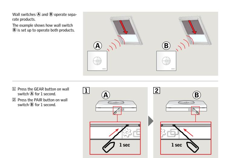
Wall switch (B) can now operate both products. Wall switch (A) can still operate its own product.
