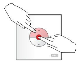
Press OPEN/UP and STOP key simultaneously for 1 second.
