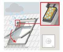
When the rain sensor is activated, the roof window will close automatically within approx. 30 seconds.
